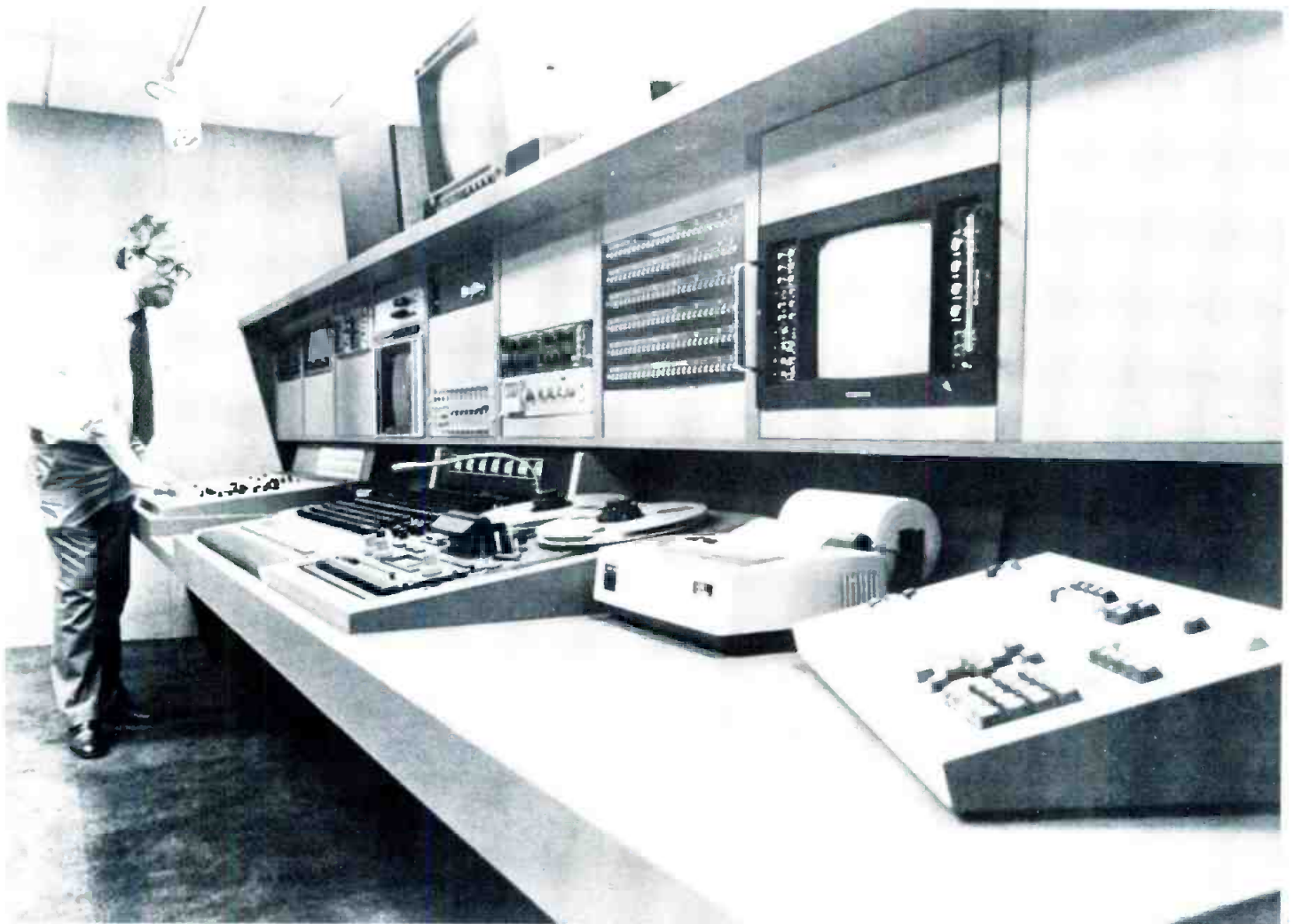
Walter Raufer, Movielab Video vice president of Engineering, checks newly-installed equipment in the new post-production facility: (left to right) Grass Valley Switches, CMX editor, AudioArts mixing console and Chryon IV character generator.
