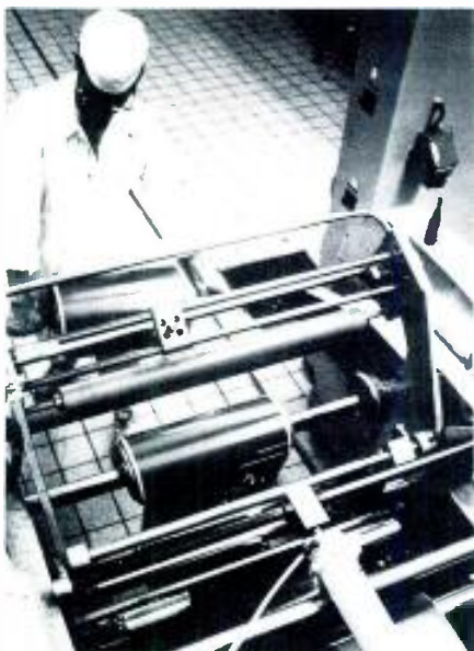
Figure 3. This machine is winding a butt roll from coated tape as it emerges from the drying tunnel.
