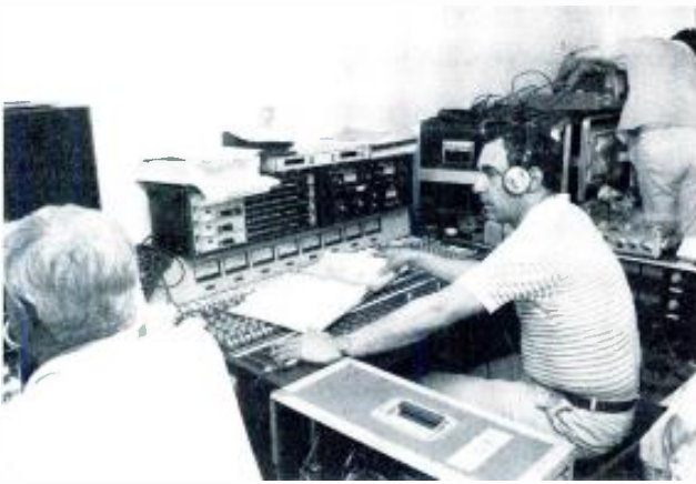
Figure 3. Ed Greene records location audio at the Audiotronics 110-8 topped by Dolbys and UREI limiters and flanked by two Otari MX-5050s.
